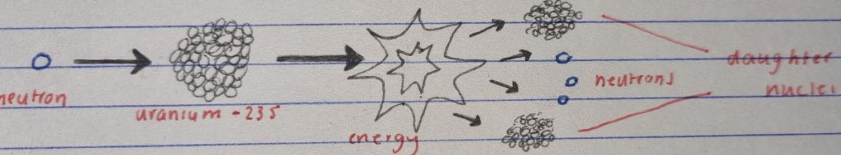
Diagram illustrating nuclear fission: A neutron ( $\circ$ ) strikes a Uranium-235 nucleus (represented by a cluster of circles). The nucleus splits into two daughter nuclei and releases energy and two additional neutrons ( $\circ$ ).
